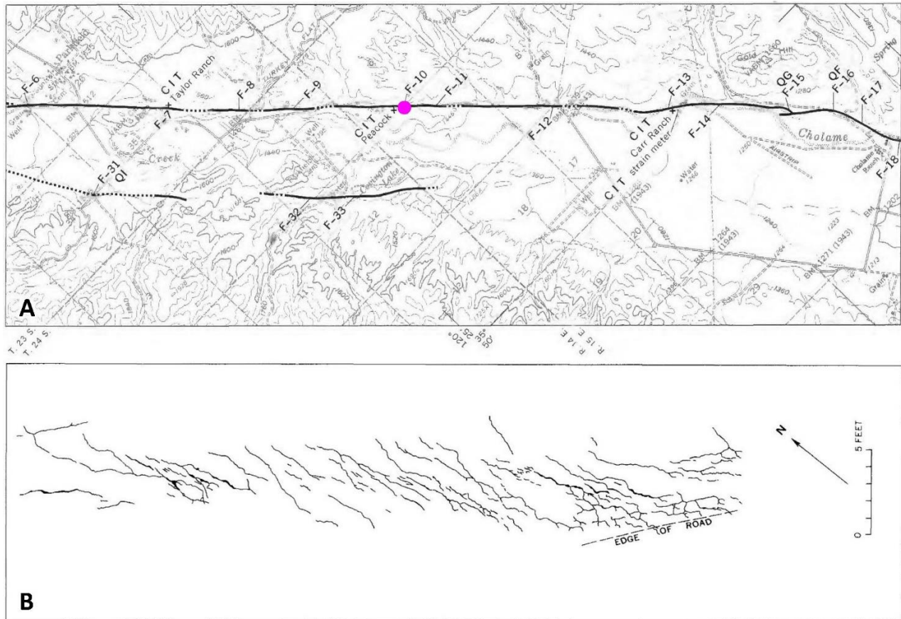
Figure 2.1. Surface rupture datasets from 1966 M 6.19 Parkfield, California earthquake. (A) Ruptures mapped on 1:24,000-scale 7.5' quadrangle topographic map; magenta dot is location F10. (B) Fractures in asphalt road mapped from vertical photographs at location F10. Source: Brown et al. (1967), USGS Professional Paper 579.
