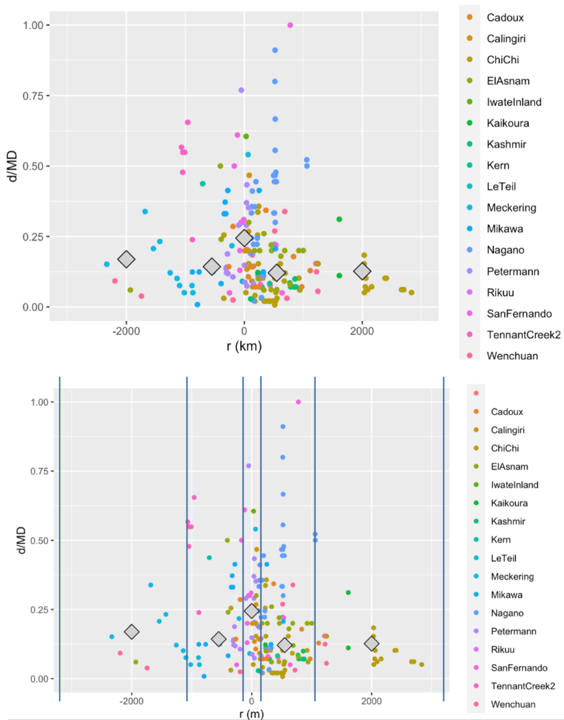
Figure 5.39. These plots show the 50 th percentiles for binned data (gray diamonds). The upper plot shows for the whole range of the data and the lower plot for the plus and minus three kilometers range. Vertical dark lines show the extents of the bins used.
