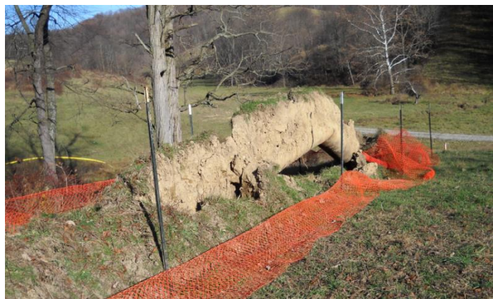
Figure 2. Examples of Upheaval Buckling Under Axial Compressive Loading
