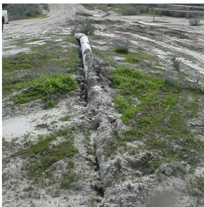
Figure 2. Examples of Upheaval Buckling Under Axial Compressive Loading
