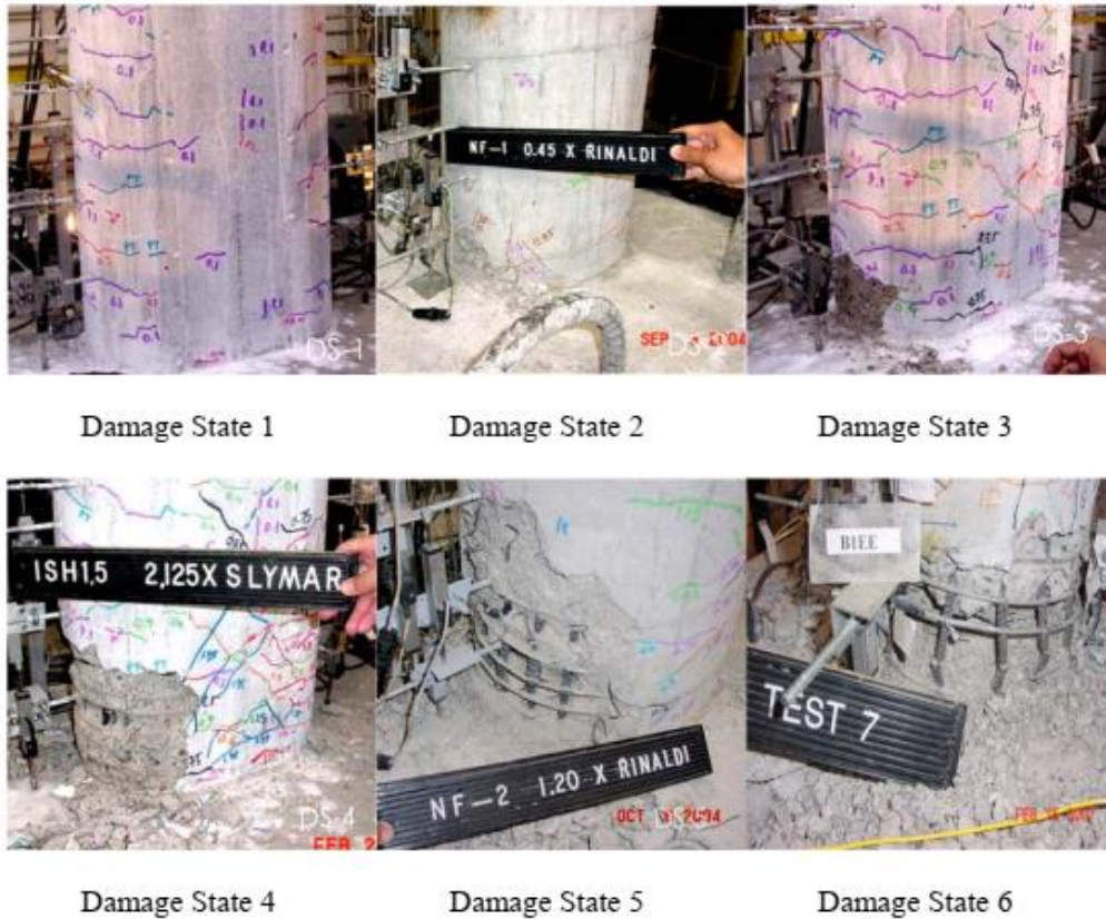
Figure 3. 10. Possible apparent damage states of bridge columns.
